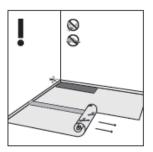
Important: installation with foil to the bottom
